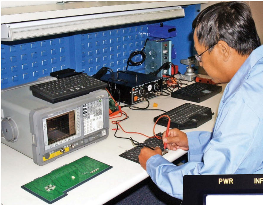
LEFT: Assembly technician Loc Bui performs final assembly testing on a custom rugged keyboard.
